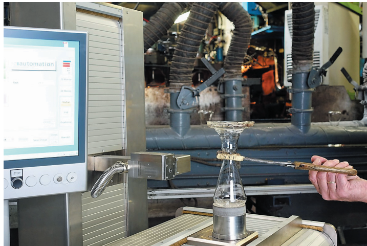
Fig. 2: Positioning a hot Erlenmeyer flask for contactless wall thickness inspection.
