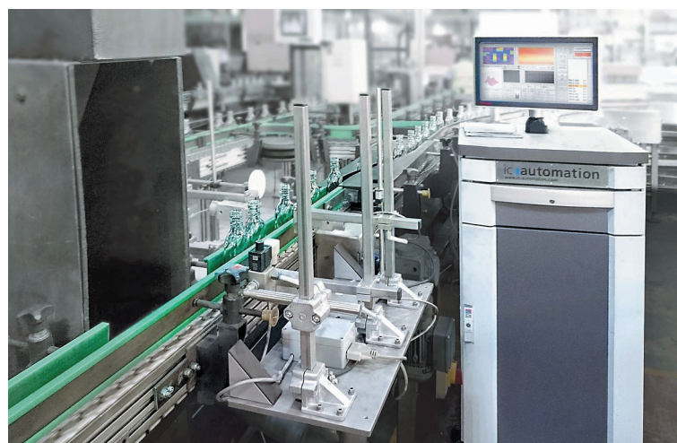
Fig. 1a (above): ICM thickness measurement on a conveyor.
