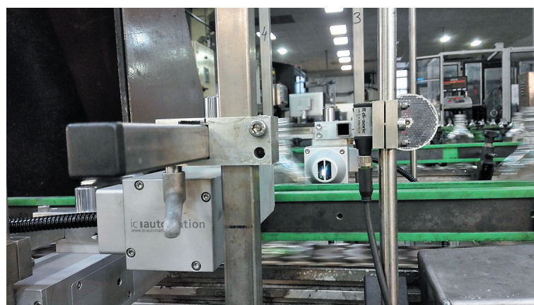
Fig. 1b (below): Robust shielded optical line probes. Photo: Allied Glass
